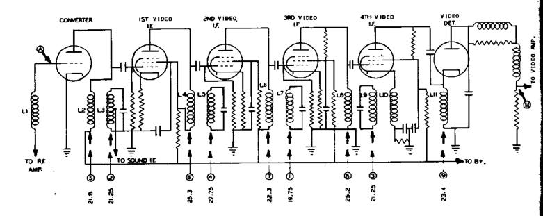
Fig. 8. Typical Stagger Tuned Video J.F. System
